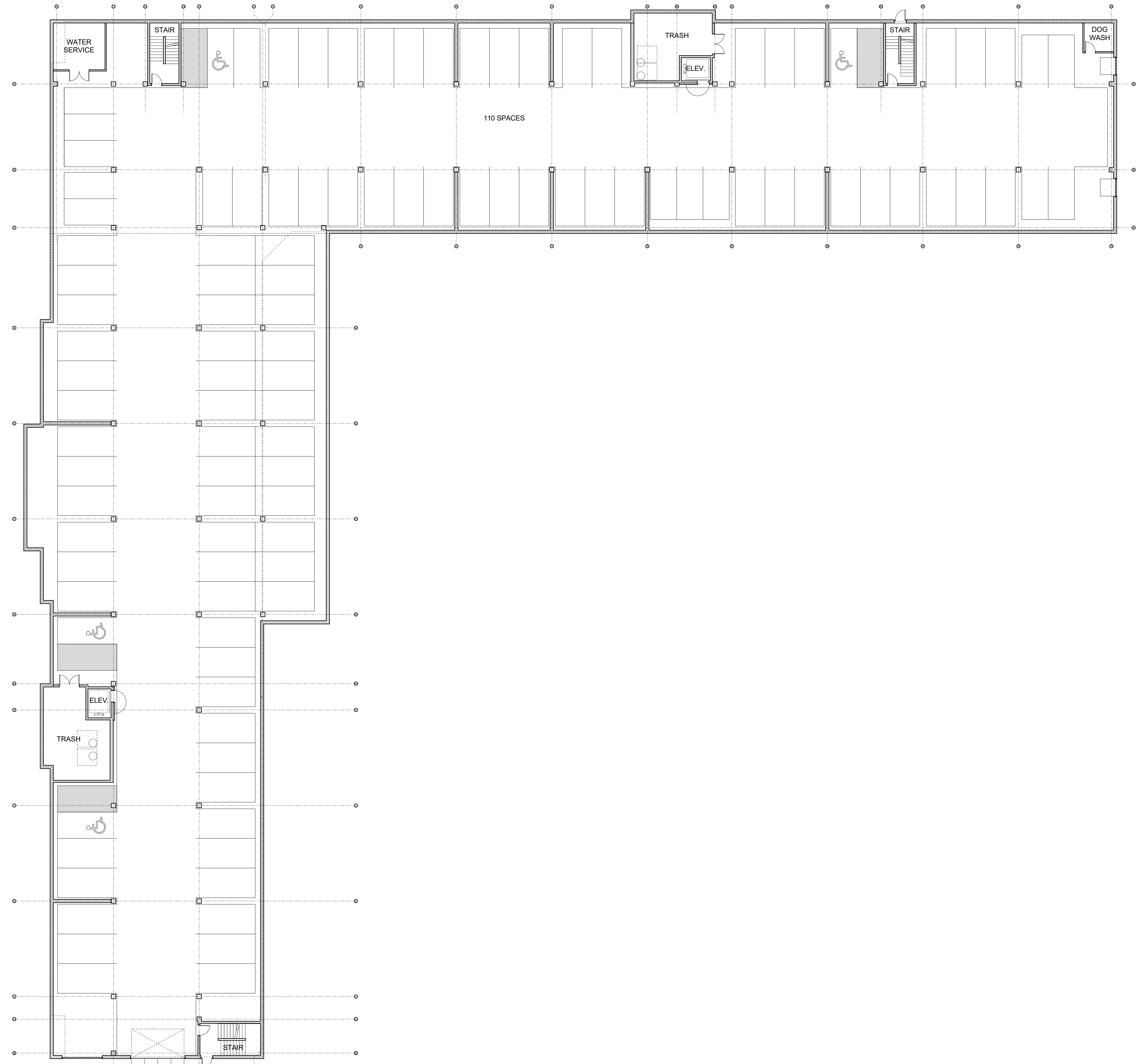
1 APARTMENT BUILDING LOWER LEVEL 1 GARAGE PLAN SCALE: 1/16" = 1'-0"
