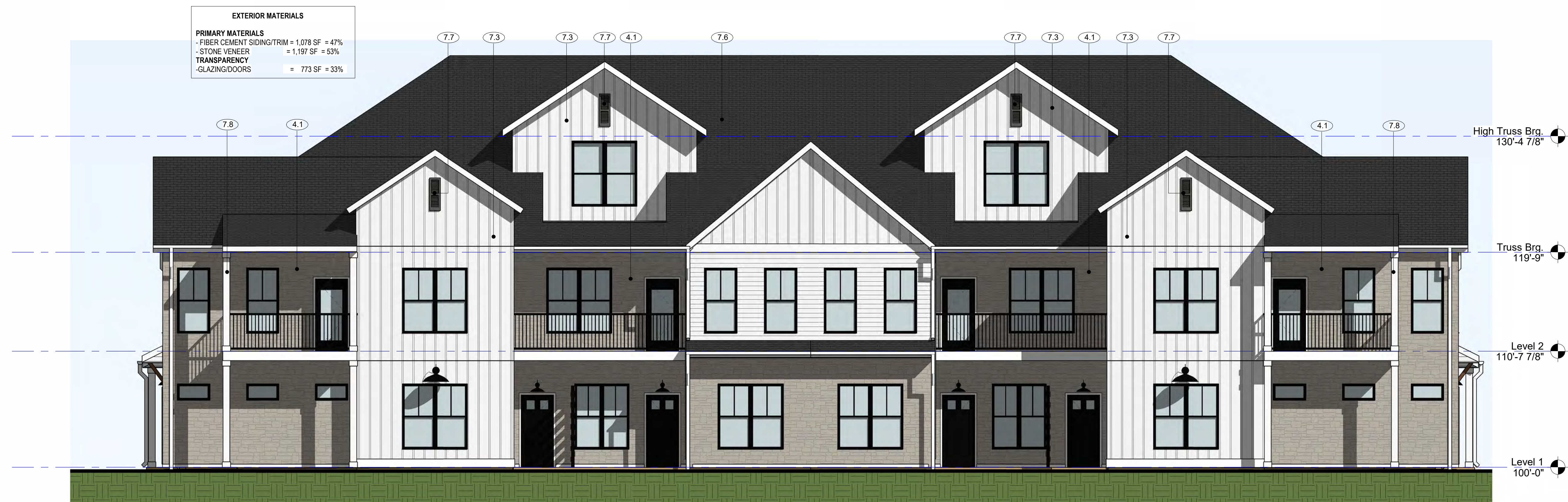
① 12-Unit Building (12A) - Front Elevation 3/16" = 1'-0"
