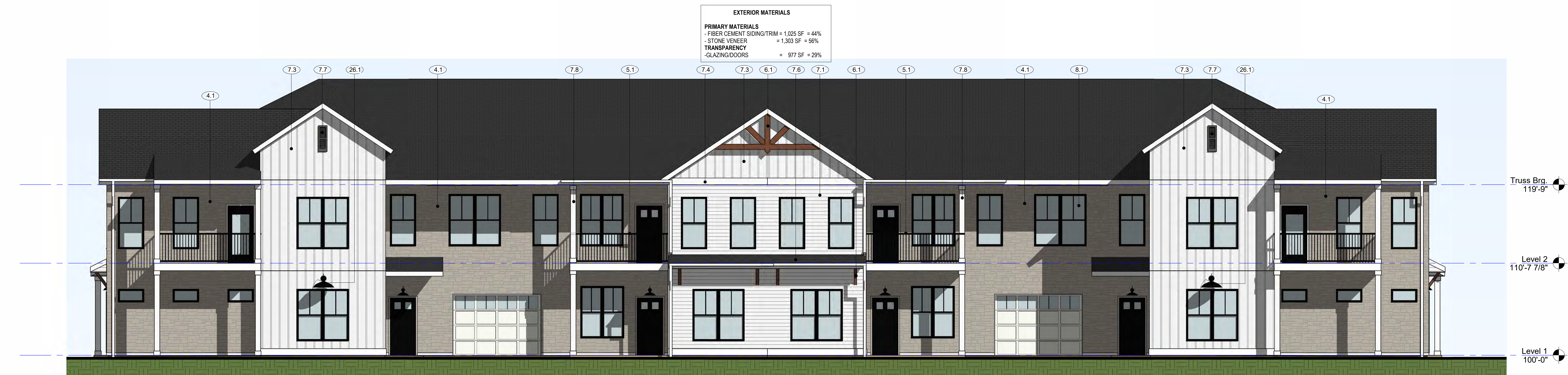
③ 12-Unit Building (Type A) - Front 3/16" = 1'-0"
