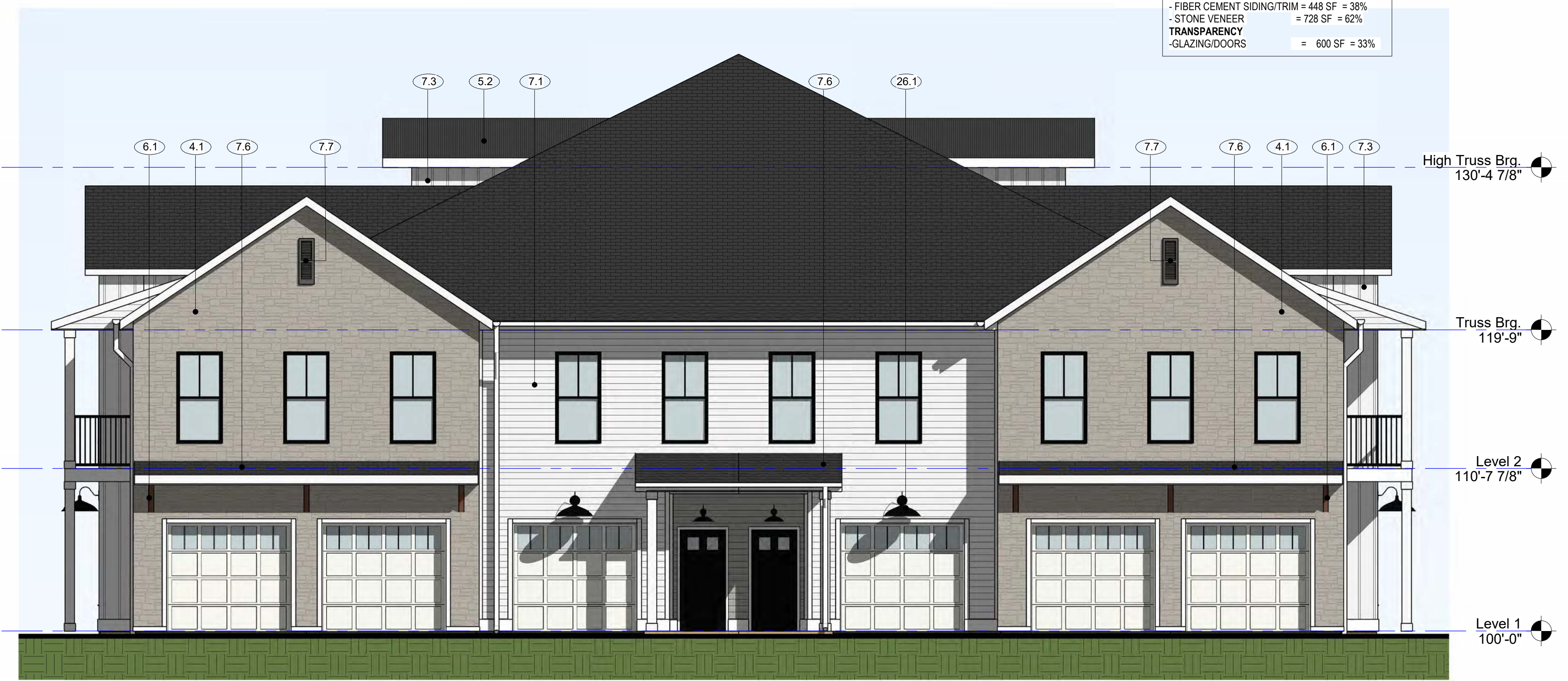
③ 12-Unit Building (12A) - Side Elevation 2 3/16" = 1'-0"
