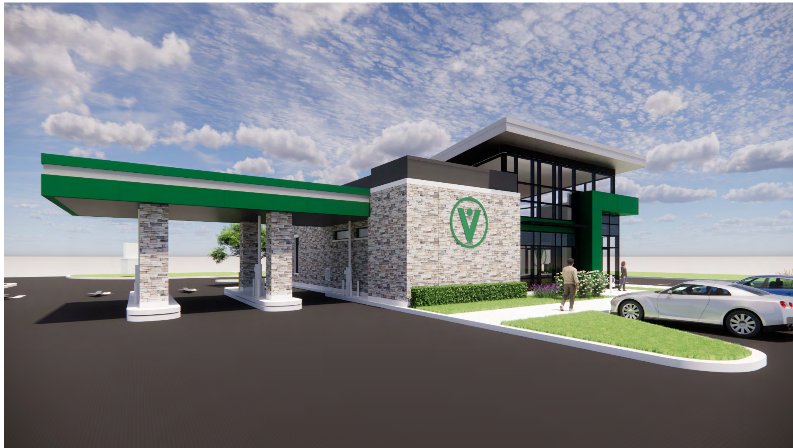
Drive-Up Canopy: Green Alpolc metal panels continue to pull the Veridian marketing colors onto the north elevation. The canopy will contain the pneumatic tubes as well as can light fixtures as well as green tape lights along the interior edge for nighttime lighting.
